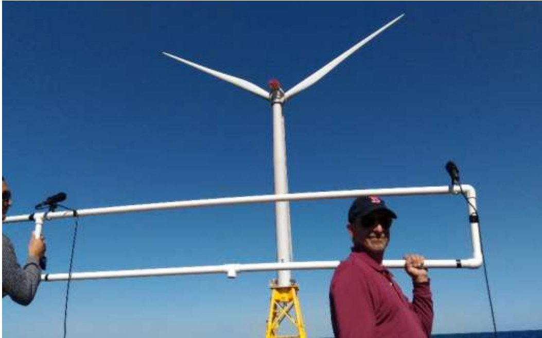
Figure 44. Customized omni-directional microphone array used for concurrent recording of air/water sound measurements.
